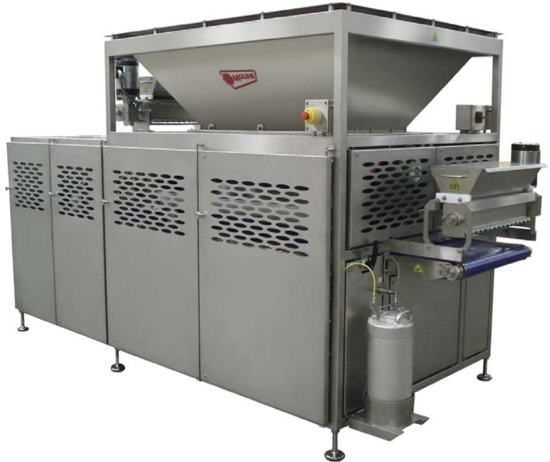
*The Moline YOGA dough sheet former is designed to deliver a true, stressless dough sheet for high-volume industrial applications. The unique three-stage design, incorporating portioning, multi-rolling and tamping/weight control, is perfect for variety bread systems, frozen or pre-fried donut systems, pizza, pita and flour tortilla lines. The unit consists of a chunker with hopper and starwheel portioning paddles, a satellite roller, tamping roller and conveyors.*
